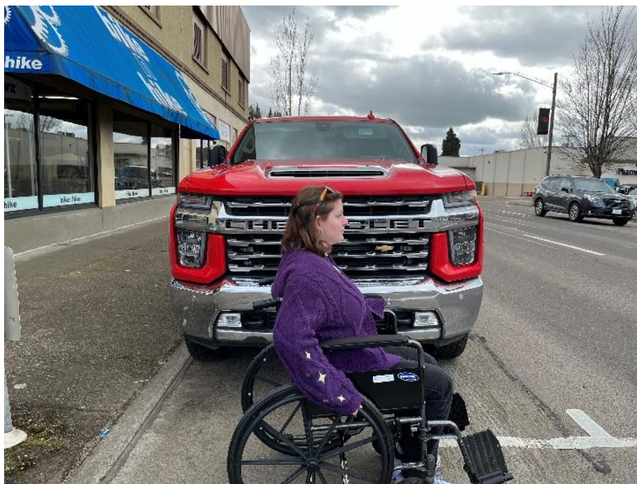
Figure 3 Pickup Hood Height in Comparison to a Person in a Wheelchair
