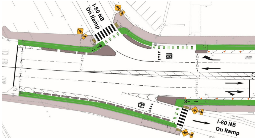
Figure 4 The On Ramp – Tight Merge at Cutting Blvd/ I-80 interchange
