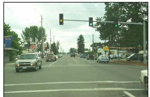
Figure 1: Four-section vertical flashing yellow arrow PPLT display in Woodburn, Oregon
