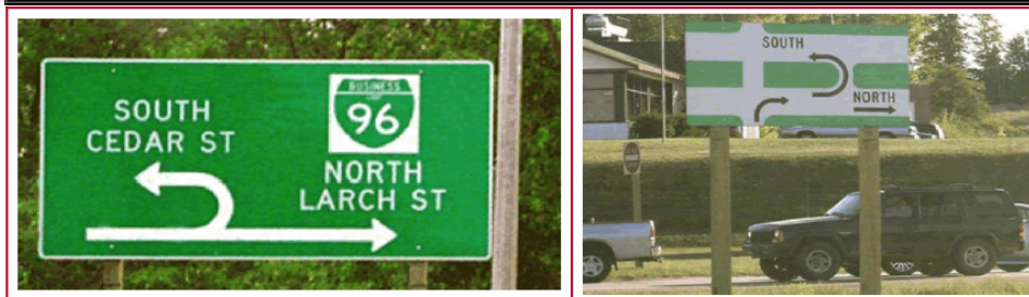
Figure 13. Examples of “innovative” signing plans for the MUTIT in Michigan.
