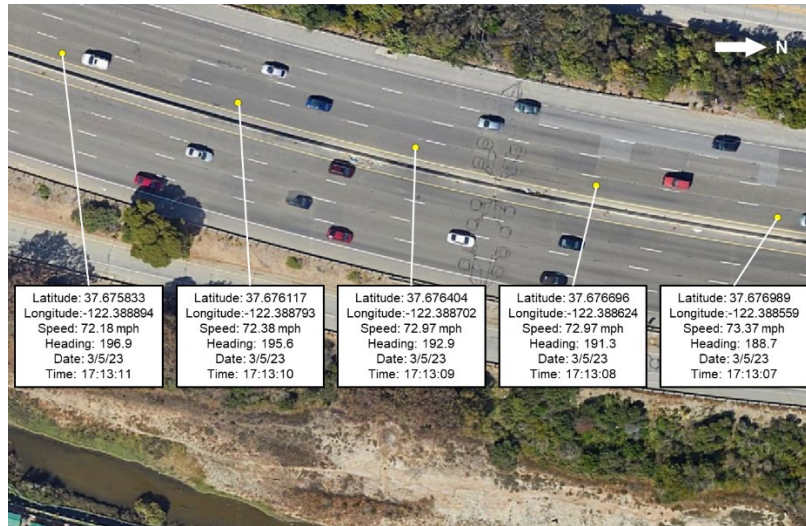
Figure 1 Part of the Continuous Trajectory Waypoints of an Individual Vehicle on Freeway Segments
