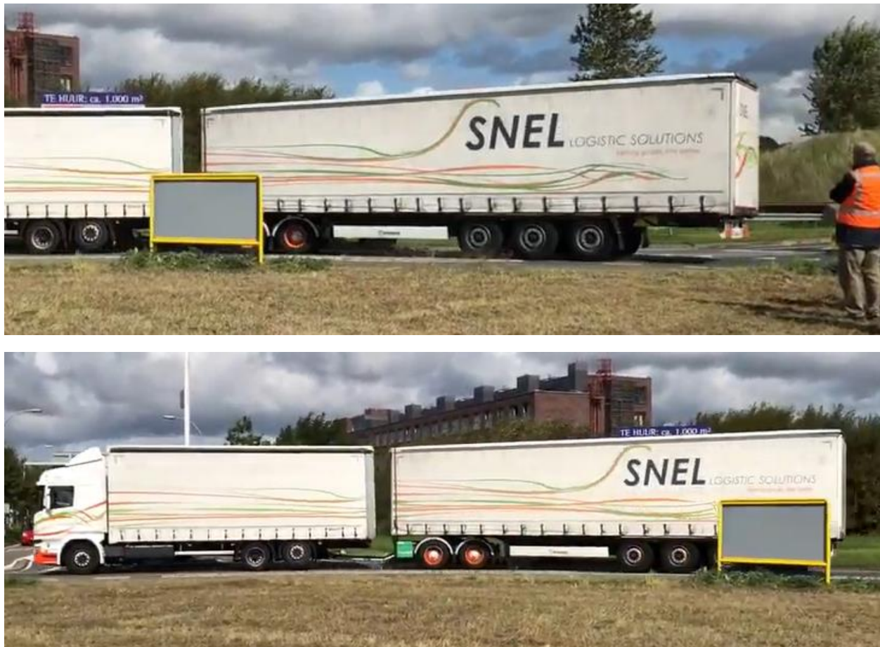
Figure 4. Still images of largest design vehicle in the Netherlands making a left turn at a Turbo Roundabout (6)
