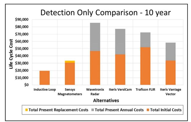
Figure 1: Detection only comparisons for 1 intersection over 10 years
