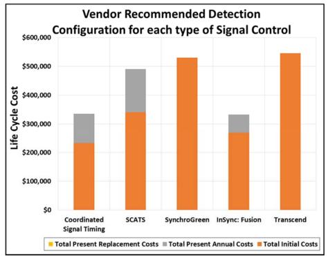
**Figure 3: Vendor Recommended Detection Configuration**
