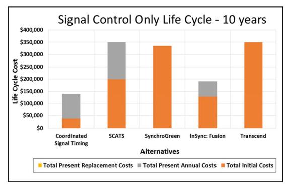
Figure 2: Signal Control Comparison for 10 year analysis
