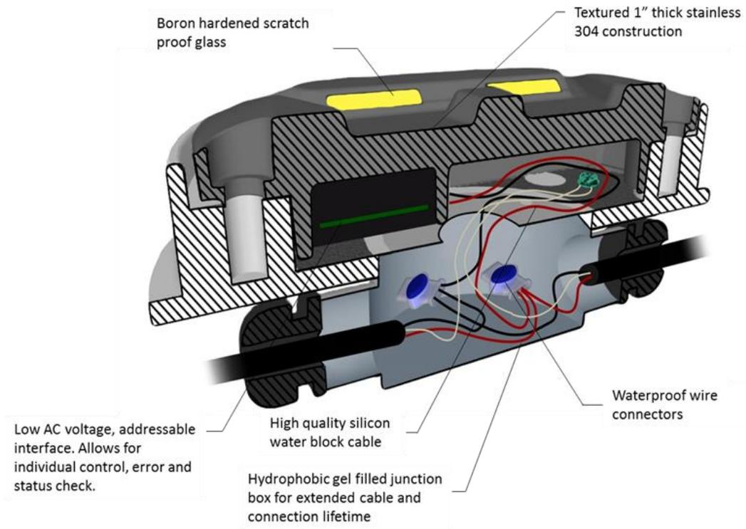
Figure 5 Section View of LaneLight™ electrical connections [6]
